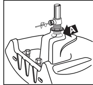
7 Return the fitted lavatory to the installed position. Connect trap to drain assembly hand tight to check alignment. It may be necessary to cut off part of the tailpiece (area "B") or part of the horizontal leg of the trap (area "C").
