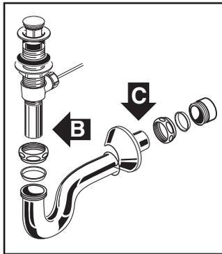
8 Secure lavatory to wall as shown in 5 or 5a. Install washers and hand tighten nuts or lag bolts. Level and square the unit. Connect hot and cold supply lines to the shut-off valves. Tighten trap joints for watertight assembly.
