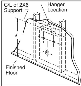
**4** Remove lavatory and pedestal from installed position. Drill pilot holes for lavatory and pedestal anchor screws or lag bolts. **Note:** Some models are supplied with lag bolts, anchor screws, or steel hangers for lavatory installations only. Other models and all pedestals are not provided with mounting hardware. Various pedestal screw sizes and types are available to the installer at local hardware outlets.
