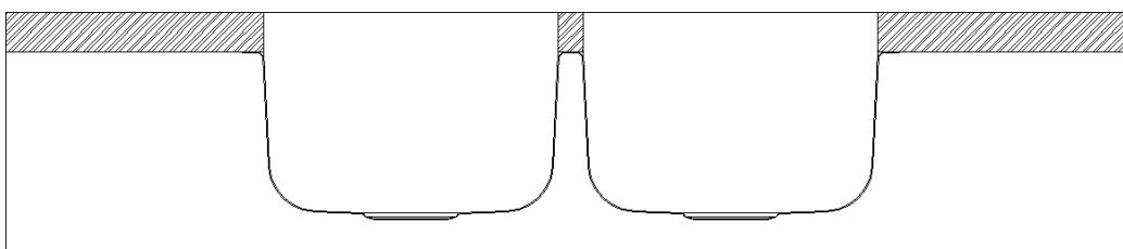
**Negative Reveal** - The counter top extends over the edge of the sink on all sides by approximately 1/4". Use caution with this installation to be sure that accessories such as colanders or cutting boards will fit properly .
